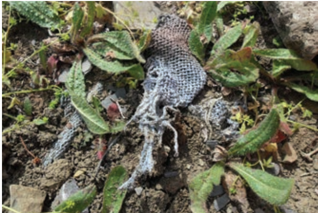
■ Figure 8. Decorative coatings containing asbestos in soil.
