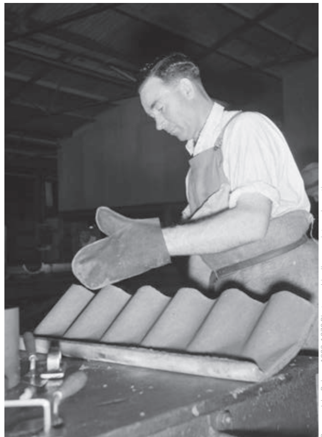
Figure 2. Manufacturing asbestos fibrolite (ca 1940s).
