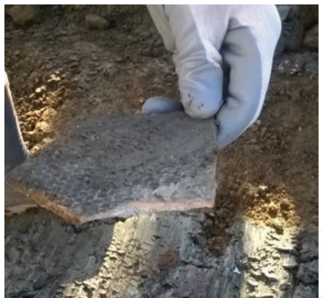
Figure 7. Asbestos-cement sheet and bonded ACM in soil.
