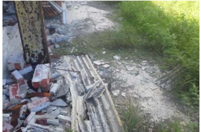
■ Figure 9. Other asbestos-containing products in soil.
