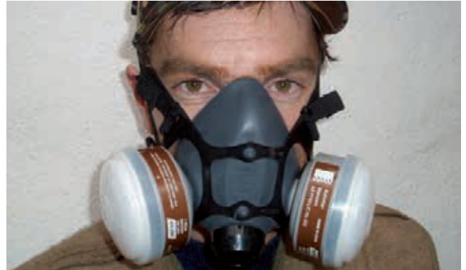
■ Half-face mask respirator that can be fitted with a P3 filter for Class B removal work.
